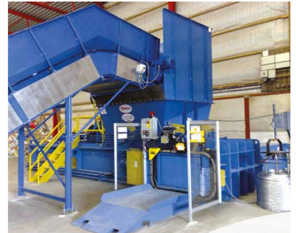
Harris Centurion baler 150 hp. Ram force 210 t. Infeed hopper 2184x2908 mm. Can be used for e.g. OCC, tyres, hard plastic, non-fe, wood, MSW.
