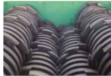
The inside of a Q65 shredder, 400 hp. 4 shafts with double hooked knives. Equipped with a sorting screen. Infeed opening 1650x1650 mm.
