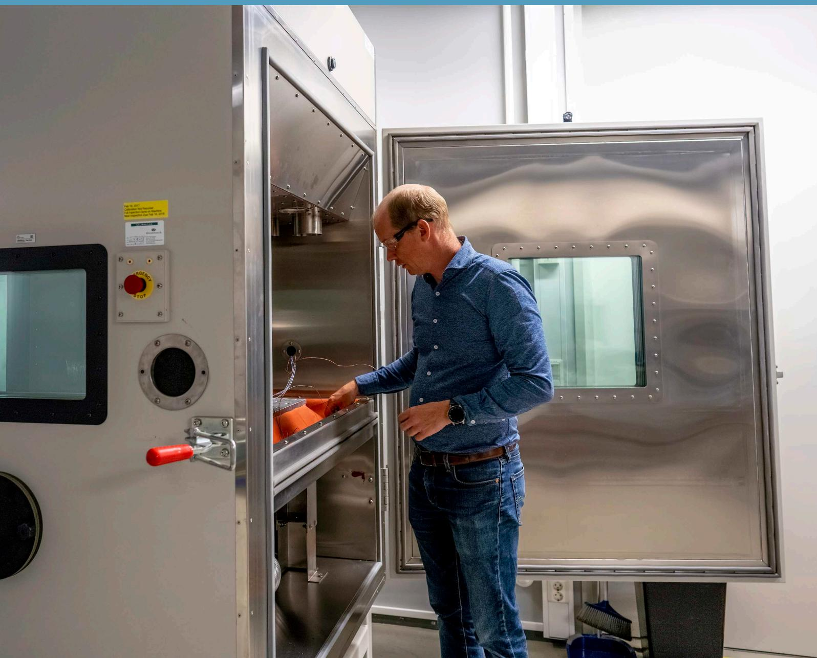
Highly Accelerated Life Tests (HALT) and Highly Accelerated Stress Screens (HASS) are designed to be a faster and more efficient way of fault finding than traditional testing methods. With HALT/HASS you can speed up the design and testing phase of your product in development and reduce failures in the field or to consumer. With robust and reliable product design, the results are savings in both time and cost.
