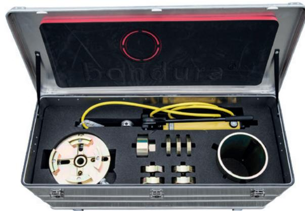
In order to simplify the removal of conical sleeves and pins we have developed a tool: bondura® Multi Tool. This is a special tool for gentle and easy removal of conical sleeves and pin - to be used on bondura® pins with diameters redundant from  $\varnothing 30$  to  $\varnothing 500$  mm.
