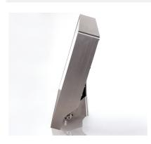
The strong 4mm bulletproof glass layer above the screen withstands acid, cleaning-and disinfectant fluids as well as extreme operational demands. Behind the glass there is a projective and capacitive touch panel. A special sensitivity control allows for reliable gesture control – and this even when wearing gloves. The slim stainless-steel chassis contains an energysaving Intel DualCore processor. The LED display allows to operate without any problems in temperature range of -35°C to +45°C.
