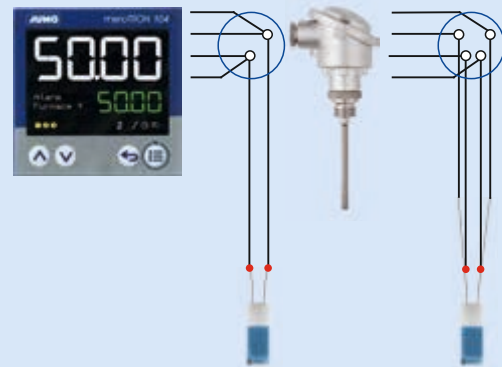
⑤ Connection of an RTD temperature probe
