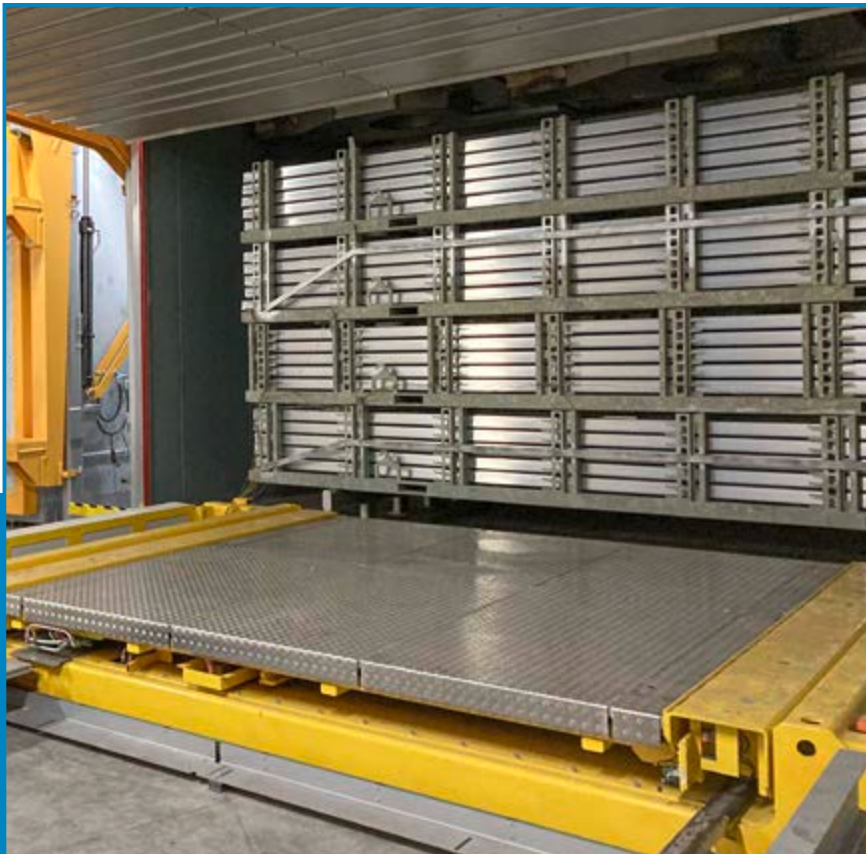
One of the 3 chamber furnaces at Aluminium-Werke Wutöschingen: Heat output: 1000 kW, Furnace size: 87 m 3 , Working volume: 43 m 3 , Calibration according to process table CQI-9
