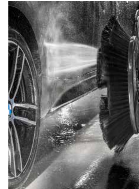
High-pressure wheel sill wash device Main soiling is removed
