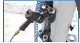
Impact wrench holder with integrated tray for support disc extensions.
