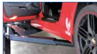
Sports car support arms with 80 mm minimum pad height (MA STAR 3.5 A Comfort).
