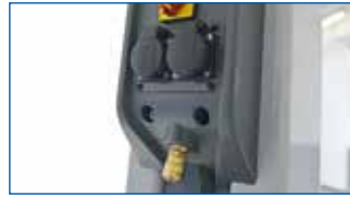
Energy set for control unit: 2 x 230 V power socket 1 compressed-air coupling
