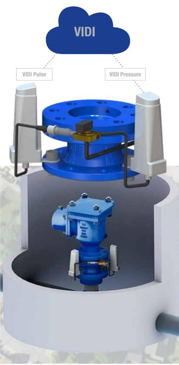
Air valves are placed on strategic places where air will accumulate, and where air pockets often occur. It is important to ensure normal working conditions for the water system; utilities do that by making sure that air valves only close after all air has left the system and water has entered the chamber.
