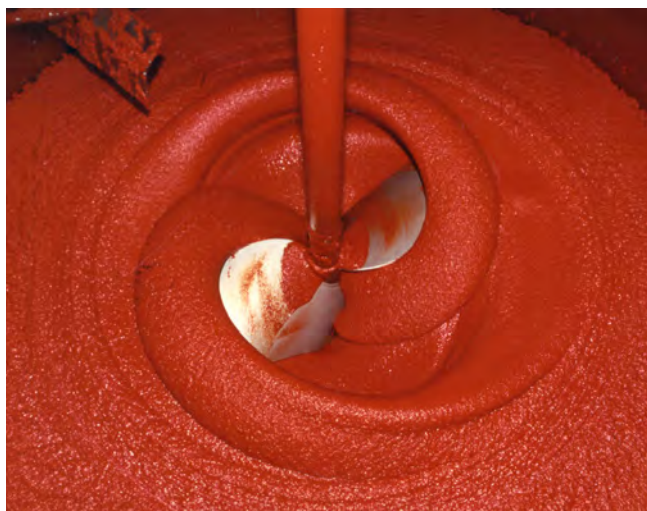
Homogenization of ketchup with a Scaba agitator with hygienic design.
