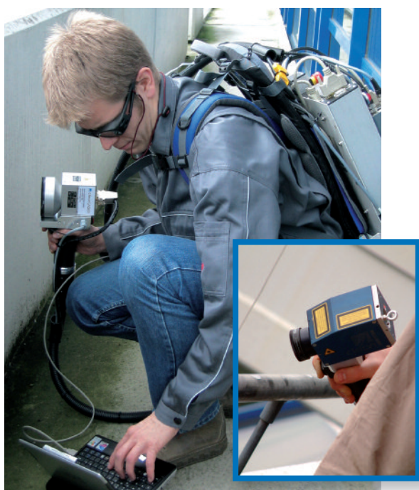
Backpack Laser in action – battery operated - no external power necessary, fiber optic beam delivery, integrated control & cooling unit
