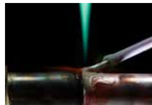
Picture 5: Clean Melting of Castolin Flux Coating
