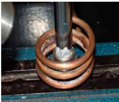
1802 HF Atmosin is formulated for use with induction processes. This flux has excellent heat resistance and does not spit or pop during rapid heating.
