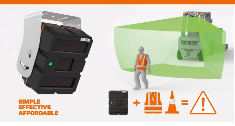
IRIS 860 sensors make pedestrian detection easy by detecting the reflective tape on high-vis safety vests and markers. If a pedestrian enters the critical risk zone they and the driver receive an audible alert.
