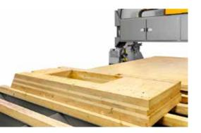
One interpolating 5-axis milling head + blade group Workable dimensions: Width from 3.000 mm up to 8000 mm unlimited length thickness up to 400 mm Graphic software specific for the walls' processing
