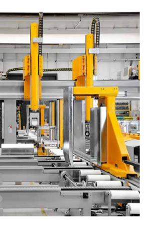
2/3 interpolating 5-axis milling head and blade group Max workable beams dimensions: 400x800 mm unlimited length Workable panels dimensions: Width from 3.000 mm up to 8000 mm thickness up to 400 mm
