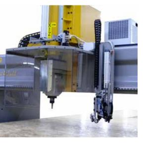
One interpolating 5-axis milling head and blade group
