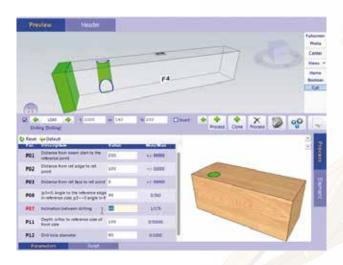
The files generated by the main CAD used for projecting are automatically converted into BTL files, which allow the immediate execution on the machine. The software installed on the TECHNO machines is provided with an OPTIMIZATION function.
