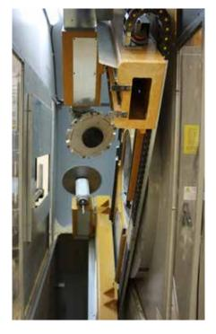
One patented "Turn" 6-axis milling head Max standard workable Beam section 650x400 mm
