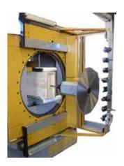
On the strong and stable portal frame is installed a precision ring nut controlled by the CN, with a 360° movement where is located the innovative "TURN" milling head.
