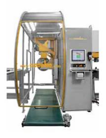
One patented "Turn" 6-axis milling head Max standard workable Beam section 240x400 mm
