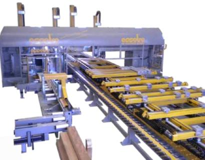
On the cross beam of the fix portal frame can be installed 2 or 3 "5- axis" milling heads equipped with free programming and HSK 63F/A tool connection and one "5-axis" head with a fix blade (max diameter 1000mm) able to cut walls and panels of big dimensions.
