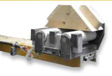
Max standard workable Beam section: 400x800mm Unlimited length
