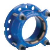
Series 623/10 Supa Plus™ flange adaptor Tensile for PE and uPVC pipes Universal drilling Ductile iron DN 40-300 PN 10/16
