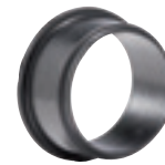
Series 05 Combi-flange sealing for uPVC, steel or ductile iron pipes Non-tensile SBR rubber DN 400-600 (uPVC and ductile) DN 50-300 (steel)
