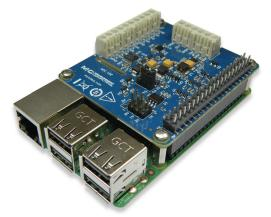
*The* MCC 152 *is a* 12-*bit analog voltage output and digital input/output* DAQ HAT. *The* MCC 152 *is shown here connected to a Raspberry* Pi (not included).
