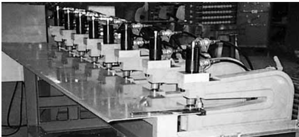
Hydraulic short-stroke cylinder to operate punching units as series punch installation.
