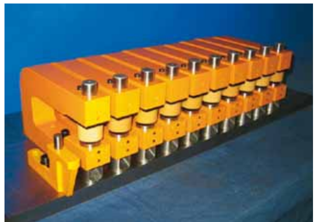
Punching units arranged with a positioning plate
