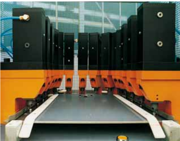
Pneumatic single-action punching units for punching shaped cuts
