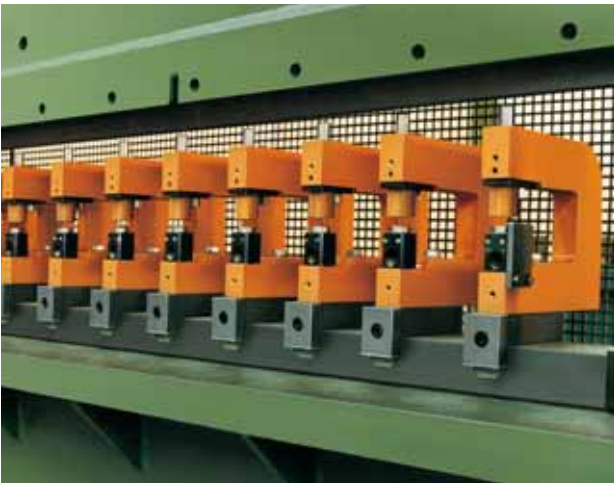
Tool units for punching in a bending press
