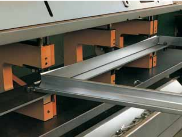
Tool units for caulking corner connections
