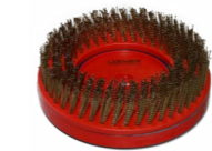
OxideDisc with angled wire brushes to remove oxide on the side edges of laser-cut steel parts.
