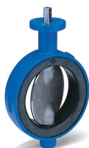
Serie 75/10 Centrisk butterflyventil Wafer Fast EPDM foring Duplex/rilsan belagt disk DN 40-300 PN 10/16 Duktijern
