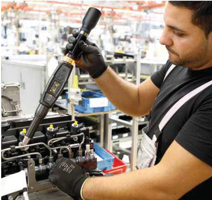
Furthermore, as the residual point is detected in real time, buzzer, LEDs and vibration alert the operator to stop, avoiding overtorqueing.
