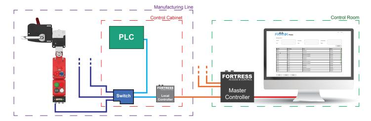
Local controller provides robustness and line-side communication
