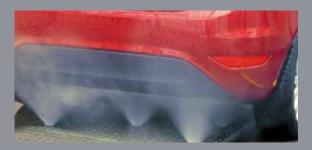
Possible choice: static underchassis wash 10 bar [145 PSI] 90 L/min [23.8 gpm], oscilating 15 bar [217 PSI] 120 L/min [31.7 gpm], or by sector 15 bar [217 PSI] 120 L/min [31.7 gpm].
