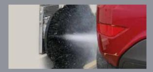
A complete car wash must include the vehicle's wheels. Available with or without high pressure; flat or spiral brushes are possible.
