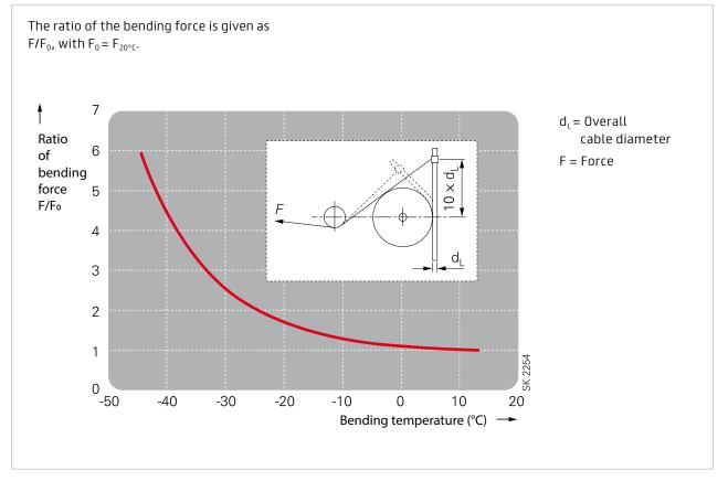
The temperature limits on the surface of the cable are specified to ensure problem-free and healthy operation during forced guidance of flexible electric cables for industrial applications, especially while trailing over ground and during reeling operation.
