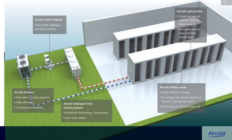
The combination of InRack server coolers that cool in closed server cabinets without mixing cold and warm air and The Intelligent Cooling System ensures minimal energy consumption for up to 350 days a year (Danish climate). Scalable, modular and redundant system design results in a high degree of f lexibility and reliability.
