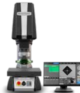
NEMESIS 5100G2 Rockwell, Vickers, Knoop & Brinell 10gf - 250 | 750 | 3000kgf
