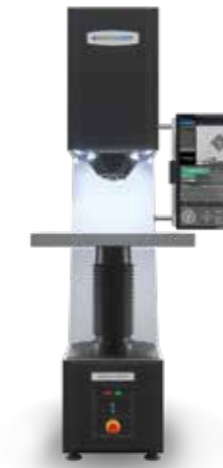
NEXUS 8100XLM G2 Rockwell, Vickers, Knoop & Brinell 200gf - 3000kgf
