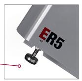
To achieve stability the ER5 has four adjustable foot stands. The rubber wheel is lifted from the ground.
