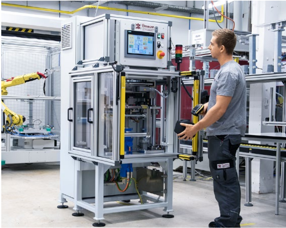
A special-purpose machine for the embossing process: the leather is positioned centrally and pressed against the embossing die from below
