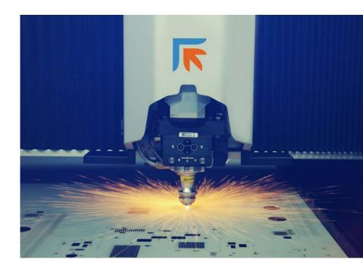
The cabin allows you to take full advantage of the **very good accessibility** offered by the cantilever structure of the machine. It is ideal when you want to process small plates loaded manually without using the pallet changer.
