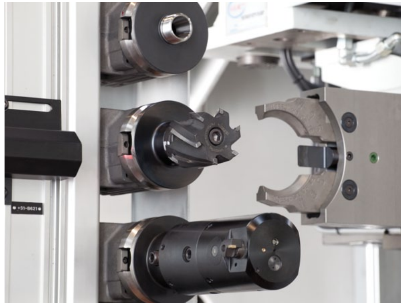
Automatic tool change from the magazine
