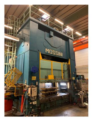
800 Ton (8000kN) Max Pressure **Bolster dimensions** 3200 x 1700 mm Slide dimensions 3200 x 1700 mm Slide adjustment 2000 mm Stroke 400 mm Stroke Speed 8-35 SPM Window (gap between housings) h x w 800 x 1050 mm Max Daylight (dist. table and slide, highest pos.) 1080 mm Overall dimensions, w x d 4700 x 2200 Height 7625 mm Weight 105 Ton With:
