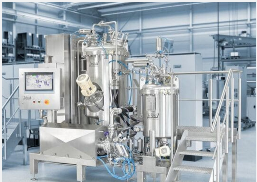
Fig. 28: ystral process plant for tablet coating production. Image: ystral
