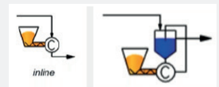
Fig. 30: Powder induction in a continuous process without (left) and with (right) ventilation. Images: ystral
