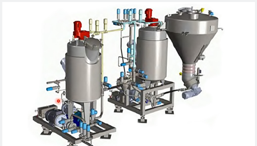
Fig. 9: Plant with two dispersing machines outside the vessels: On the left, an inline dispersing machine for the production of emulsions, on the right, a Conti-TDS for the processing of powders. Image: ystral
