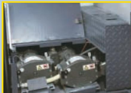
*Installed on the UV varnish tower coater of MAN Roland R700 series printing presses, twin baseplate-mounted 701 pumps have reduced downtime and increased production speed. One pump accurately metres the water-based varnish from a container to a weir on the press, the other scavenges excess varnish for re-circulation.*
