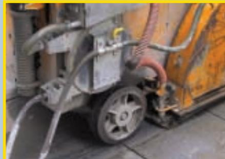
*Watson-Marlow Bredel peristaltic pumps are used wherever quality and reliability are paramount – as here, powering coolant flow in a concrete-cutting machine in Japan. The pump is the circular housing, centre.*
