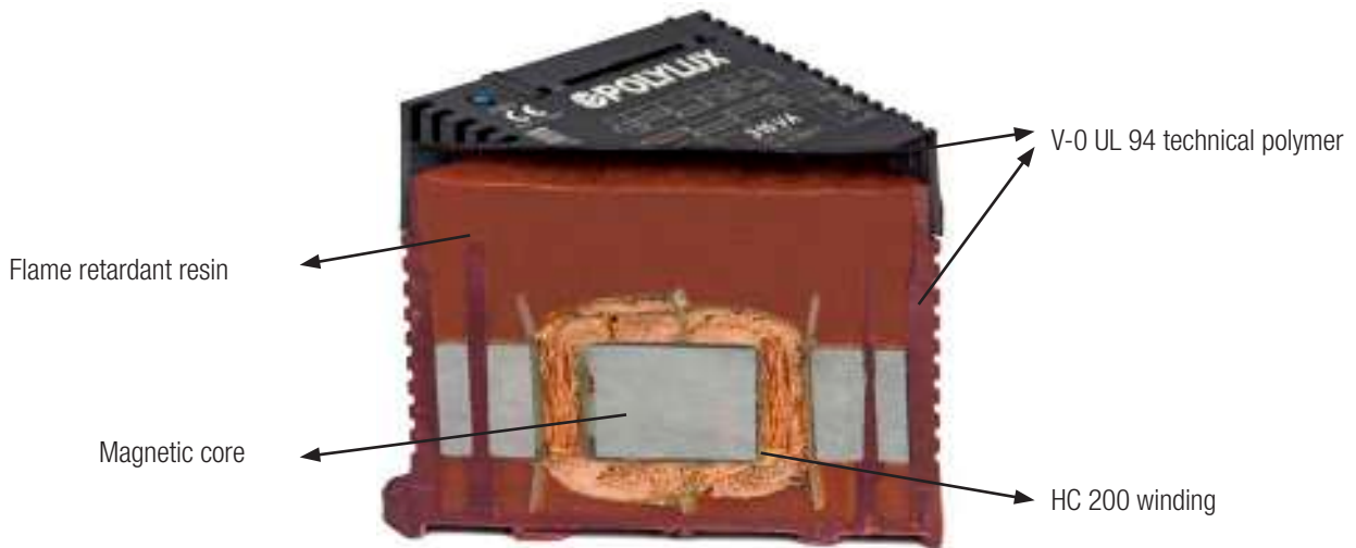
Sectioned transformer
