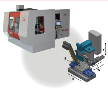
X= 1200 mm Y = 725 mm Z = 350 mm Deep drilling diameter Ø = 5-30 mm W = max .depth 1150 mm
