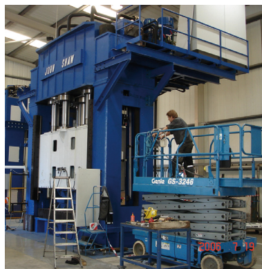
Hydraulic Upgrade, July 2006 A John Shaw press is undergoing final inspection and testing by Hydraulic staff after a complete upgrade at the FRANKE company W & G Sissons Ltd. – a UK-based enterprise manufacturing steel sinks, catering equipment, and sanitaryware.
