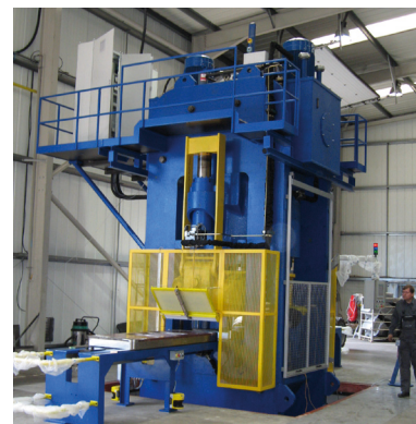
Hydraulic Upgrade, August 2006 A 5500T rubber pad press at the FRANKE company W & G Sissons Ltd. is almost ready for production testing after an upgrade. The press had been severely damaged in a fire at the factory a few months earlier.
