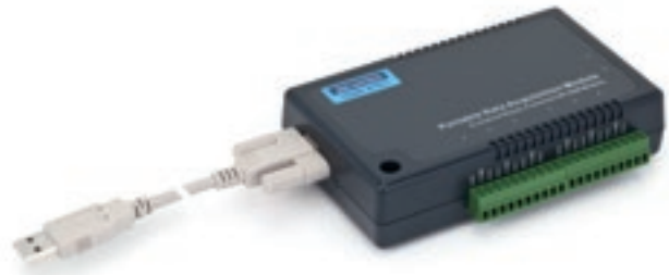
USB relay box (Art. no. 10450-1-0174) for processing various fan status messages.
