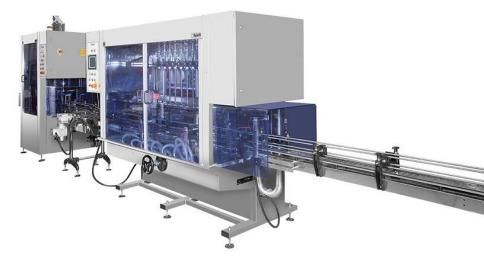
electrical cabinets and HMIs allow for non-intrinsically safe electrical components to be situated away from unsafe areas, whilst galvanic isolation allows for intrinsically safe electrical signals to enter and exit ATEX zones safely.
