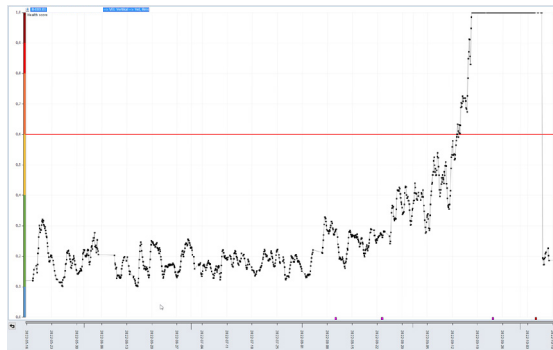
The Health score shows a sharply rising trend before the bearing replacement.
