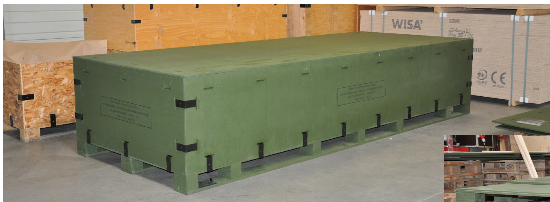
The Clip-Lok box above holds a 300 cubic meter fuel bladder. Box dimensions are 3836 x 1486 x 818 mm. When the fuel bladders are not in use they can be collapsed and stacked minimizing the space required to store them. This box is painted with NATO Green IR inhibitor paint.
