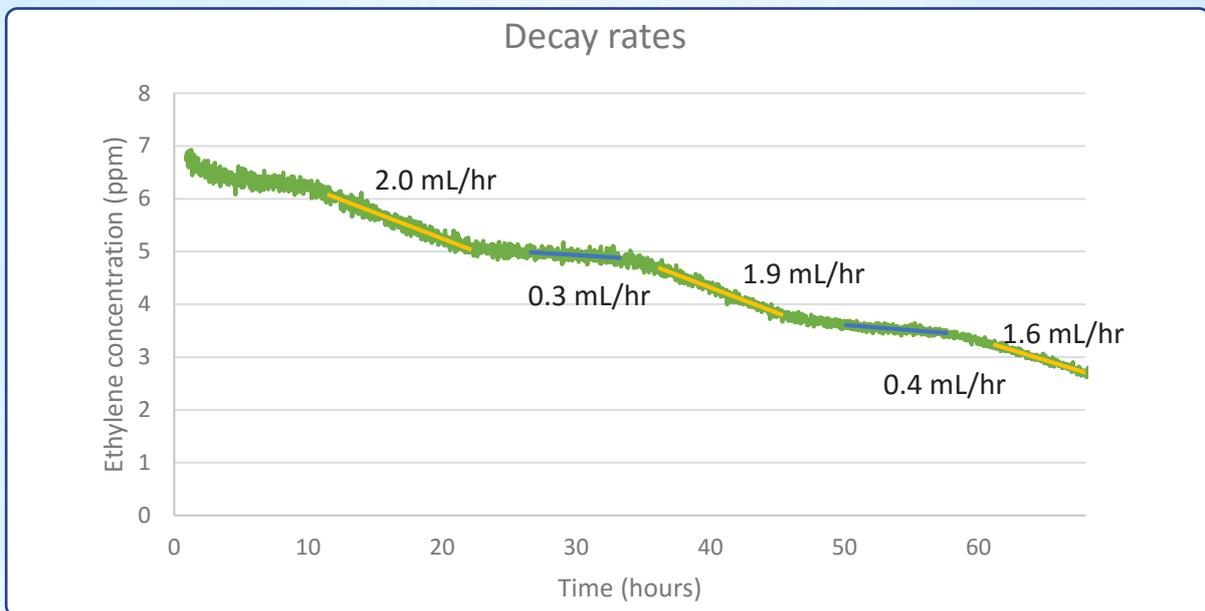
*Decay rates in milliliter per hour determined for when the air cleaner is on (yellow) or off (blue).
