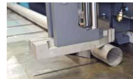
Automatic program controlled clamping pressure reduction via proportional valves for the processing of thin wall tubes and special profiles.
