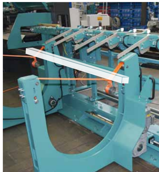
3 Section cross distributor with cross beating chains for automatic sorting of cuts forwards and backwards.
