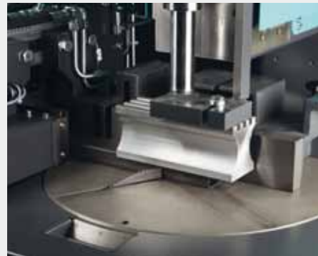
Material clamping on both side of the saw blade; work piece stop for bilateral mitre cuts.
