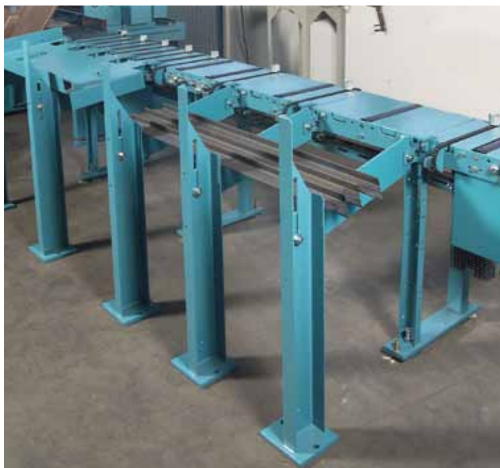
2 Automatic lowering bell troughs for the support of sections.
