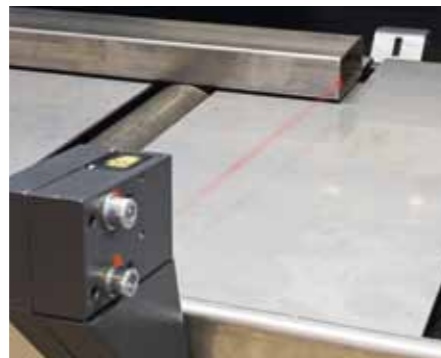
Laser light barrier for the cut identification.
