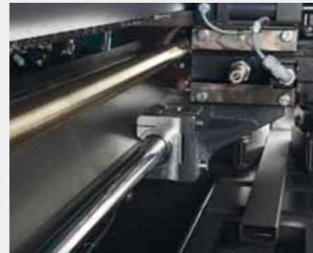
Automatic material supply via ball screw.
