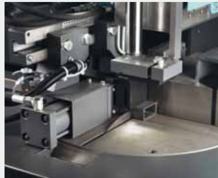
Adjustable work piece stop for 90° cuts and short residual parts lengths in automatic mode.
