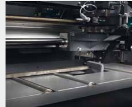
Mechanical cut stop for material identification.
