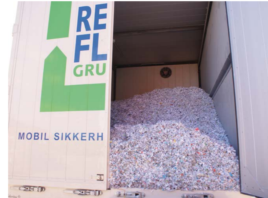
The paper is shredded and mixed into the locked cargo room with a capacity of approx. 5-6 tons shredded paper. The output material fulfills DIN norm 66399 security level P3/P4 through the mixing and the screen size of the shredder.
