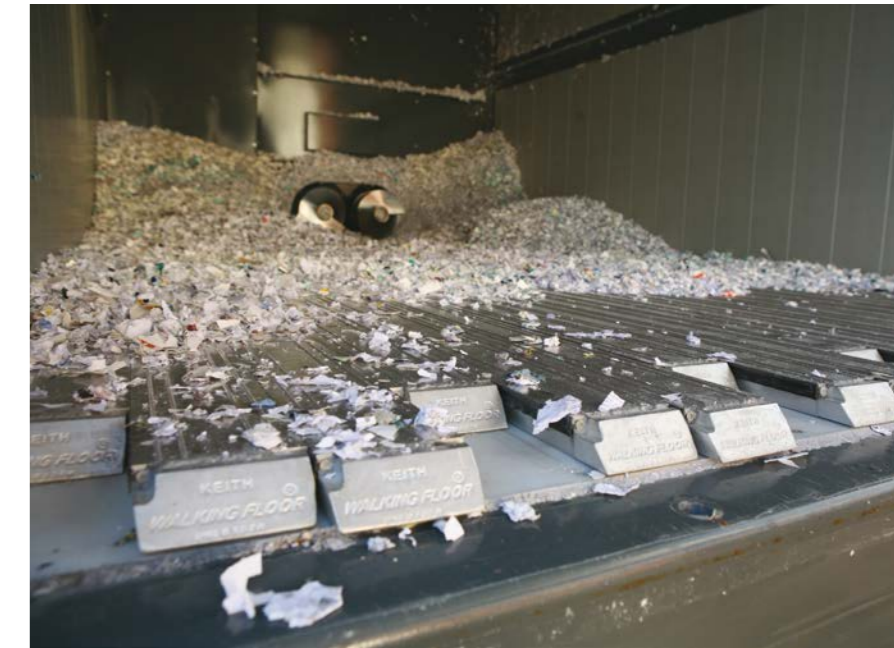
Unloading backwards with a Walking Floor.
