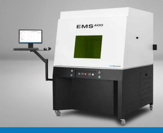
With the ability to run up to four axes, EMS400 is ideal for large tray and part marking. EMS400 features an automated XY stage, ideal for marking trays of parts or large components in multiple locations. A front vertical pneumatically actuated door maximizes operator ergonomics. The system can be controlled without a PC using the included operator hand-held control pendant.
