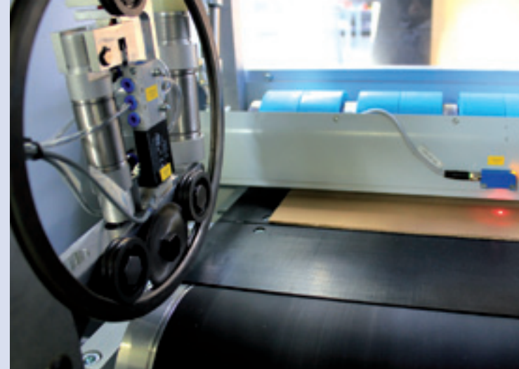
Wear-free zero-edge trimming cut
