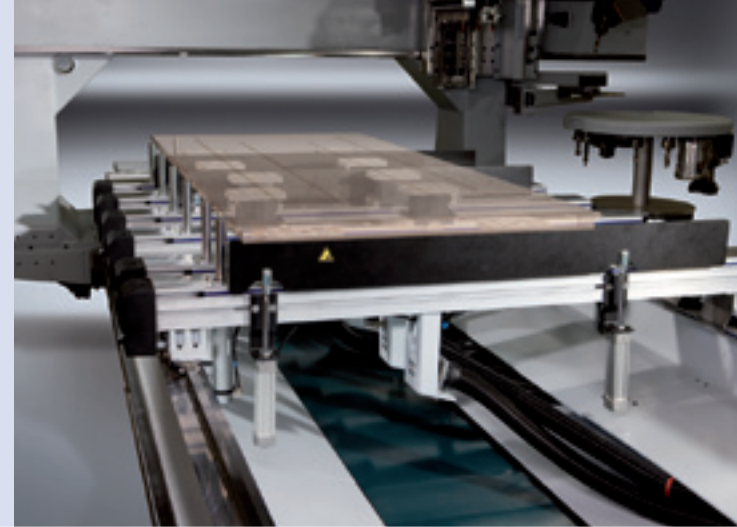
Panel material is held in position by suction for efficient vacuum production.
