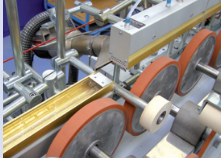
The parabolic heater provides precision heating with no loss due to dissipation
