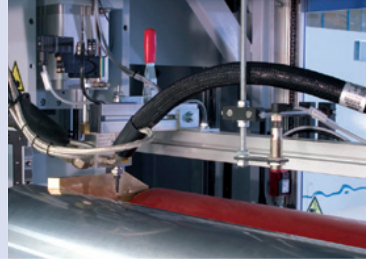
Compression jaw system of a PWR composite panel unit
