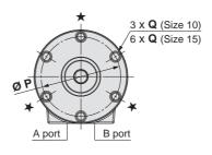
(3 mounting holes with the  $\bigstar$  marks are for tightening the actuator and not to be used for external mounting for size 10.
