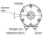
☆Recommended tightening torque for hexagon nut to fix the adjustment bolt Size 20: 1.5 N·m Sizes 30, 40: 3 N·m
