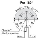
\*1 For size 10, the tolerance of rotating angle of 90° and 180° will be +5°.
