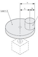
Example: 1 If the load is divided into the 2 cylinders: The centre of gravity of load 1 matches the shaft The centre of gravity of load 2 differs from the shaft Obtain the moment of inertia of load 1:
