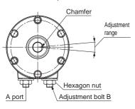
2. Set the adjustment bolt A while supplying pressure from the B port.
