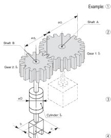
Example: 1) Obtain the moment of inertia I1 around shaft A:
