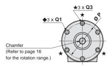
(3 mounting holes with the ★ marks are for tightening the actuator and not to be used for external mounting for size 10.
