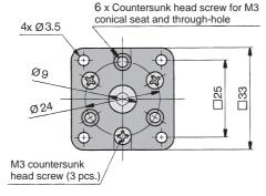
Flange assembly for size 20 Part no.: P211060-2
