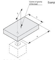
Example: 1) If the load is the thin rectangular plate: Obtain the centre of gravity of the load as I<sub>1</sub>, a provisional shaft.
