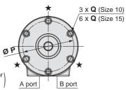
(3 mounting holes with the ★ marks are for tightening the actuator and not to be used for external mounting for size 10.
