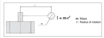
This formula represents the moment of inertia for the shaft with mass m, which is located at distance r from the shaft.
