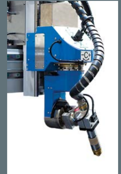
With totally +140 and 330 degrees moving area at C axis, has a 470 degrees moving and operation area in total.
