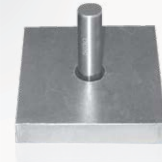
12 mm hole cutting without True Hole Technology
