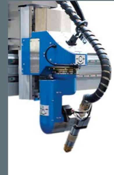
Can move totally 180 degrees at A axis.
