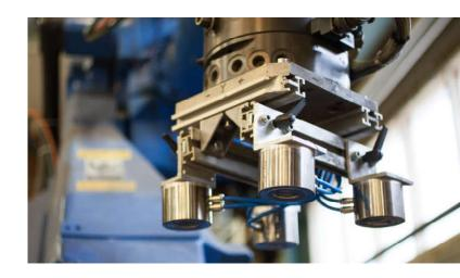
MAP-6, MAP-40 and MAP-180 magnets are especially designed for flat parts that fully cover the magnet's gripping surface. The magnets can also be used with narrow loads and perforated materials, but the gripping force is lower.
