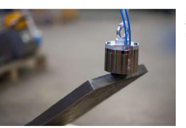
MAP-120R and MRP-130F magnets' gripping surfaces are optimized for parts that do not fully cover the whole gripping surfaces of the magnets.
