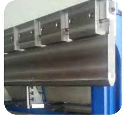
Heavy-duty clamping system up to 350t/m (optional)
