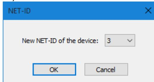
Figure 273: NET-ID dialog box used to assign a NET ID when adding a new base device
