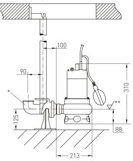
\* Elbow supplied by customer \*\* Lowest switch-off level (lowest switch-on level is at least 100 mm higher)
