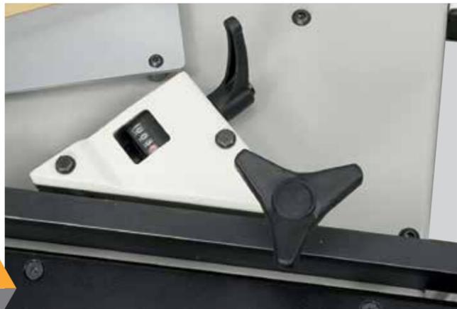
Entry guide with micrometric adjustment according to the edging thickness. The edging thickness to be applied is shown by a decimal numerical indicator.
