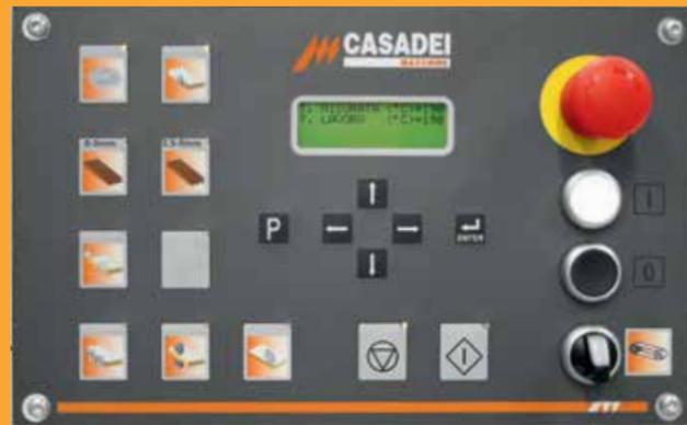
Control panel positioned at the machine's infeed in an ergonomical position. The whole machine and all working units present (apart from the edge scraping unit) are controlled by PLC.
