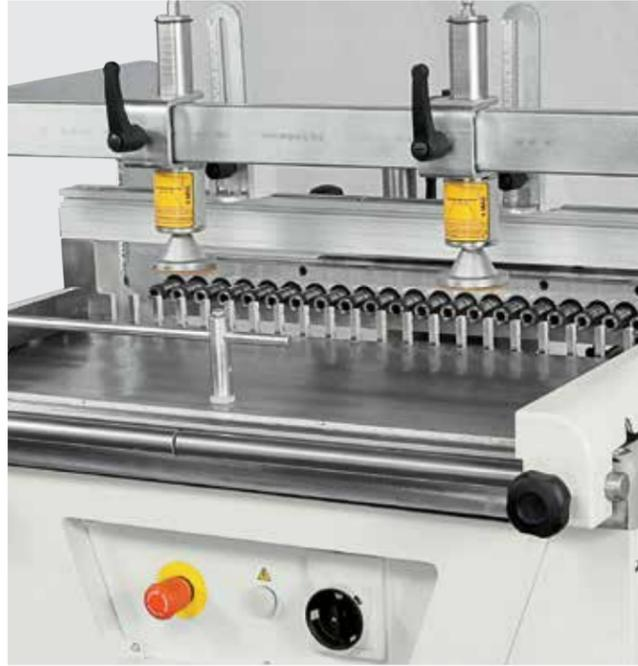
Reference compass for positioning the guides in specular mode (standard).
