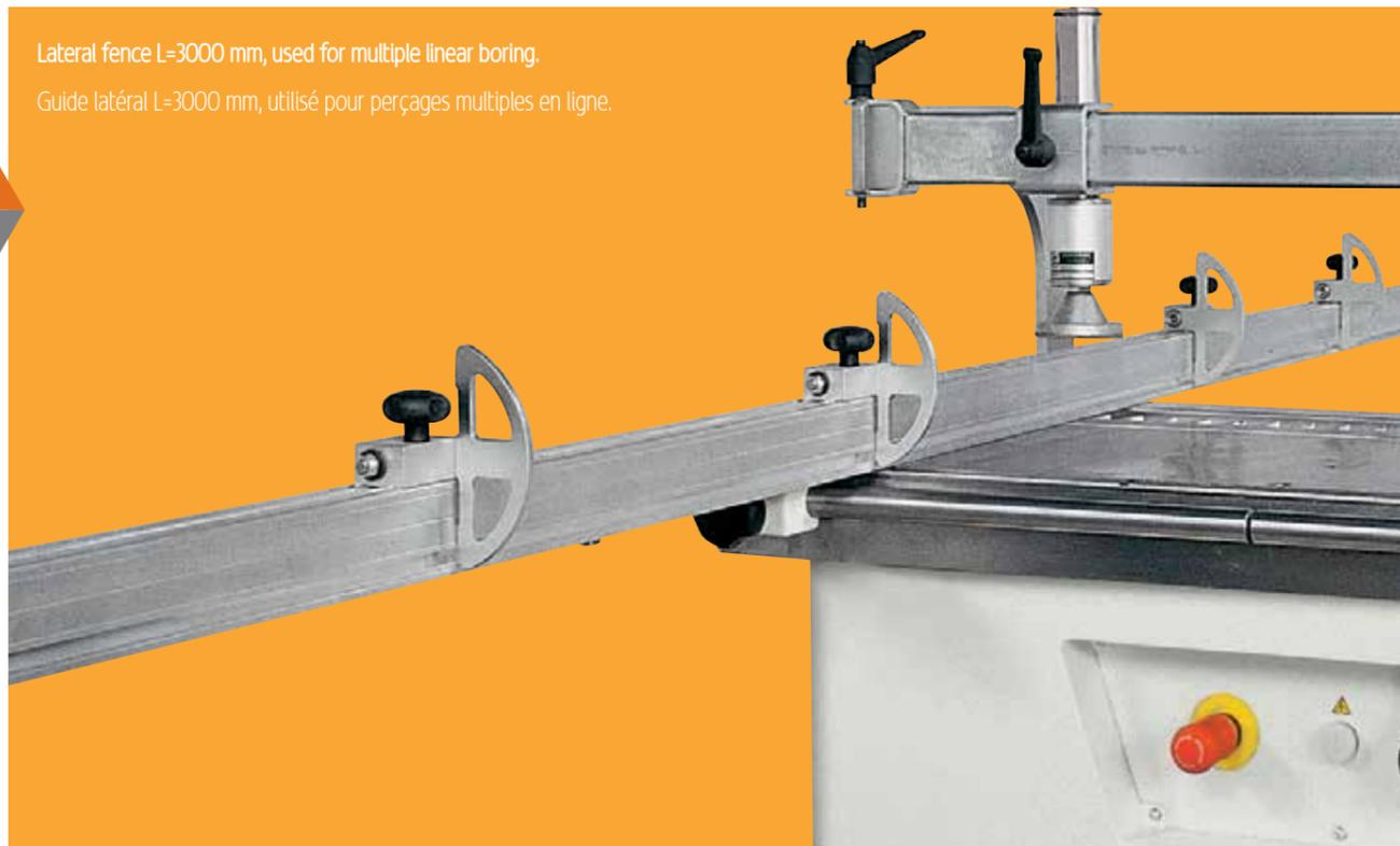
Lateral fence L=3000 mm, used for multiple linear boring.
