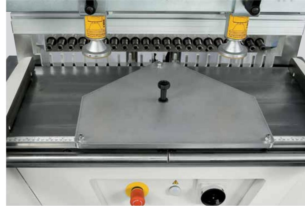
Fence for horizontal boring at  $\pm 45^\circ$ , normally used for  $90^\circ$  joints.
